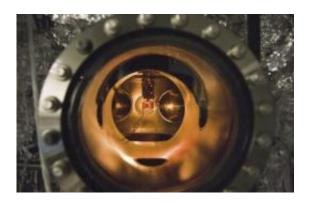
A small PETE device made with cesium-coated gallium nitride glows while being tested inside an ultra-high vacuum chamber. The tests proved that the process simultaneously converted light and heat energy into electrical current. Credit: Photo courtesy of Nick Melosh, Stanford University
