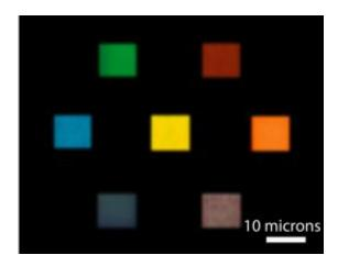
An optical microscopy image of seven color filters illuminated by white microscope light. Credit: Jay Guo
