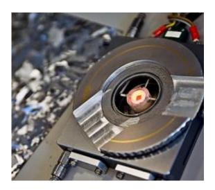
A tiny silicon chip — the glowing orange square at the center of this special heating device — is heated to a temperature well below silicon's melting point, and then very slowly cooled down. The chip inside this heating device was placed in the path of a synchrotron beam to probe its changes at a molecular level as it went through the retrograde melting process. Photo: Patrick Gillooly
