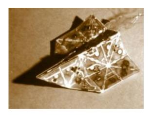
Studded with magnets and electronic muscles known as actuators, a prototype robot developed at MIT can automatically fold itself into an airplane or an origami boat.
