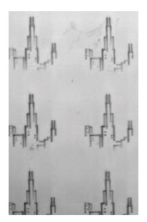
Using beam-pen lithography, Northwestern researchers patterned 15,000 replicas of the Chicago skyline simultaneously over square centimeters of space in about half an hour.
