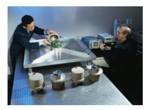
Dr. Richard Blakeslee (right) and Tony Kim (left) of the Marshall Center test the electric field mills used to measure lightning produced by thunderstorms. (NASA/MSFC/D. Stoffer)
