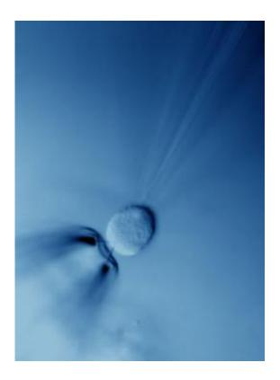
This is an optical image of a two-terminal nanowire nanoprobe internalized by a single cell. The device has a three-dimensional and flexible structure with the key nanoscale field-effect transistor element synthetically-integrated at the tip of the acute-angle nanowire nanostructure. 3-D nanoprobes modified with phospholipid bilayers enter single cells in a minimally-invasive manner to allow robust recording of intracellular potential. Credit: Courtesy of Charles Lieber, Harvard University
