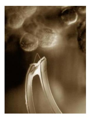
This shows the delivery of a two-terminal nanoscale transistor sensor into single cells. The device has a three-dimensional and flexible structure with the key nanoscale field-effect transistor element synthetically-integrated at the tip of the acute-angle nanowire nanostructure. 3-D nanoprobes modified with phospholipid bilayers enter single cells in a minimally-invasive manner to allow robust recording of intracellular potential. Credit: Courtesy of Charles Lieber, Harvard University.
