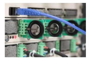
The metallic disks are experimental batteries being tested in the Laboratory for Energy Storage and Conversion run by NanoEngineering professor Shirley Meng at the UC San Diego Jacobs School of Engineering. Photo credit: UC San Diego
