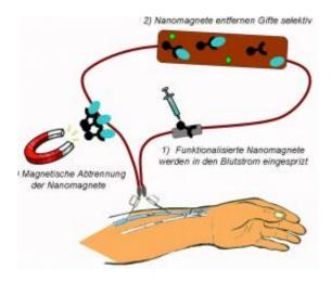
The illustration shows how the nanomagnet purifier works. (Picture: ETH Zurich)
