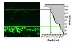
A 3-D nanofluidic "staircase" channel with many depths was used to separate and measure a mixture of different-sized fluorescent nanoparticles. Larger (brighter) and smaller (dimmer) particles were forced toward the shallow side of the channel (fluorescence micrograph on left). The particles stopped at the "steps" of the staircase with depths that matched their sizes. Credit: S.M. Stavis, NIST
