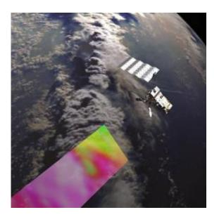
MetOp-A is Europe's first polar orbiting satellite dedicated to operational meteorology, and with its contribution to the American Polar Orbiting Environmental Satellite (POES) Programme it marks a new era in global weather prediction and climate monitoring. From its polar orbit 800 kilometres above the surface of the Earth, MetOp's range of European and American instruments will provide a wealth of accurate and detailed information to meteorologists and scientists around the world.
