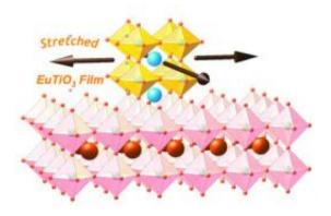
Cornell researchers made a thin film of europium titanate ferromagnetic and ferroelectric by "stretching" it. They did it by depositing the material on an underlying substrate with a larger spacing between its atoms.
