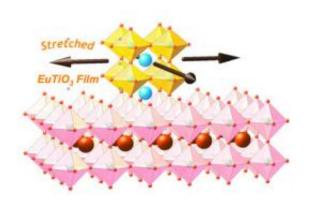
Cornell researchers made a thin film of europium titanate ferromagnetic and ferroelectric by "stretching" it. They did it by depositing the material on an underlying substrate with a larger spacing between its atoms.
