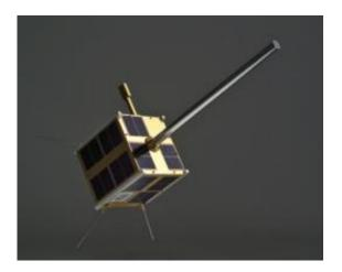
The first Norwegian satellite developed in Norway, AISSat-1 was launched on 12 July 2010. It is being used to detect AIS signals from ocean-going traffic in conjunction with a comparable experiment aboard ESA's Columbus module of ISS. Credits: Norwegian Space Centre
