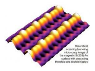
This is a theoretical scanning tunneling microscopy image of the magnetic Si(553)-Au surface with coexisting threefold and twofold ripples. Credit: Naval Research Laboratory
