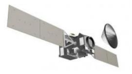
This is an artist's impression of the ESA/NASA ExoMars Trace Gas Orbiter. The orbiter will carry a European entry, descent and landing demonstrator vehicle. Credit: ESA
