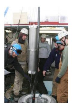
IceCube scientists deploy a calibration light source, called the Standard Candle in one of the 2.5 km deep holes. Each of the 86 holes contains a string of 60 Digital
