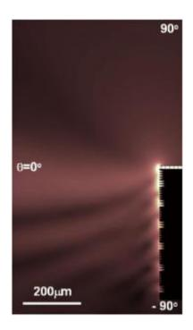
The deep "pink" grooves form an effective grating that coherently scatters the energy of the surface waves into the far-field. Credit: Courtesy of the laboratory of Federico Capasso, Harvard School of Engineering and Applied Sciences
