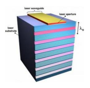
The metamaterial patterns are directly sculpted on the highly doped GaAs facet of the device. Artificial coloring in the figure indicates deep and shallow micron scale grooves, which have different functions. The shallow "blue" grooves efficiently couple laser output into surface electromagnetic waves on the facet and confine the waves to the facet. Credit: Courtesy of the laboratory of Federico Capasso, Harvard School of Engineering and Applied Sciences
