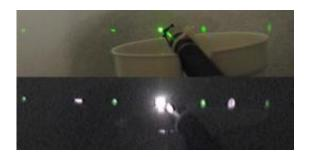
IR leakage: (Top) Photo from an ordinary camera shows light from a green laser diffracted into several spots. The green laser pointer is visible in the foreground. (Bottom) The same vignette photographed by a webcam with no infrared-blocking filter reveals intense diffraction spots from 808nm infrared light, invisible to the eye. Credit: NIST
