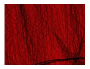
This is a colorized micrograph of the world's darkest material -- a sparse "forest" of fine carbon nanotubes -- coating a NIST laser power detector. Image shows a region approximately 25 micrometers across. Credit: Aric Sanders, NIST
