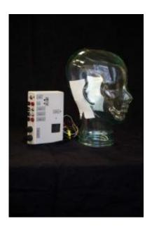
The Galvanic vestibular stimulation (GVS) system delivers small amounts of current to a person's vestibular nerve, mimicking the sensorimotor disturbances that can affect an astronaut's ability to walk and stand and impact their ability to land a spacecraft, making it an excellent tool to train astronauts before missions. Mount Sinai School of Medicine's Dr. Steven Moore leads this National Space Biomedical Research Institute-funded project. (Photo courtesy of Eric Wolfe Photography.)
