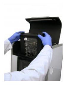
Inserting a loaded disposable cartridge into the Integrated DNA Forensic Analyzer for DNA fingerprinting of a buccal swab sample.
