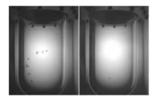
Bell jars in the Chicagoland Observatory for Underground Particle Physics consist of a steel vessel that contains the fire-extinguishing liquid iodotrifluoromethane (CF3I). Scientists would expect to see a weakly interacting massive particle leave a single bubble, like the one at right, when it hits the nucleus of an atom in the CF3I molecule. Other types of charged particles would leave multiple bubbles, like the ones at left. Credit: Fermilab
