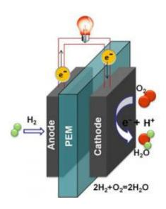
Fuel cells work by electrochemically decomposing fuel instead of burning it, converting energy directly into electricity.
