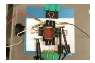
This is a prototype of the vertical stack multi-color electrowetting display device is shown in the photograph. Arrays of ~1,000-2,000 pixels were constructed with pixel sizes of  $200 \times 600$  and  $300 \times 900$  µm. Credit: American Institute of Physics
