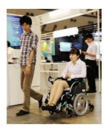
A robotic wheelchair, developed by Saitama University's professor Yoshinori Kobayashi, follows or moves beside a walking person automatically during a demonstration at the Robotech exhibition in Tokyo. Robotic wheelchairs, mechanical arms and humanoid waiters are among the cutting-edge inventions on show at a robotics fair in Japan, a country whose population is ageing rapidly.
