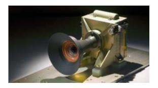
This Mars Descent Imager (MARDI) camera will fly on the Curiosity rover of NASA's Mars Science Laboratory mission. Image credit: NASA/JPL-Caltech/Malin Space Science Systems
