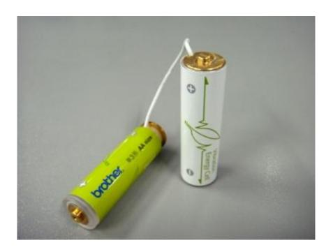
In this AA-size prototype, the generator and rechargeable battery are installed in two different cases. The voltage of the capacitor is 3.2V or lower. Image credit: Brother Industries Ltd.
