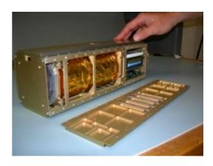
The insides of a standard nanosatellite. Credit: NASA Ames
