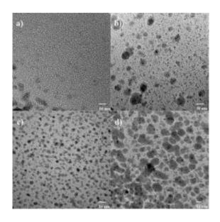
Electron microscope images of the coatings which show the silver nanoparticles incorporated in the matrix as dark spots.
