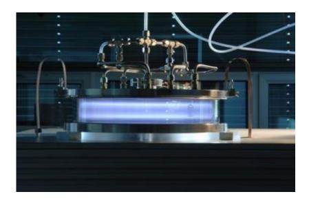
A high-frequency plasma reactor in which the nanocomposite coatings are
