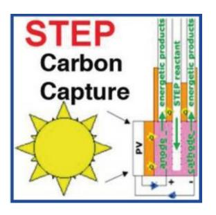
In the Solar Thermal Electrochemical Photo (STEP) carbon capture process, the sun's visible light and heat are used to capture large amounts of carbon dioxide from the atmosphere and convert it to solid carbon for storage or carbon monoxide for fuel generation. Image copyright: Stuart Licht, et al. ©2010 American Chemical Society.
