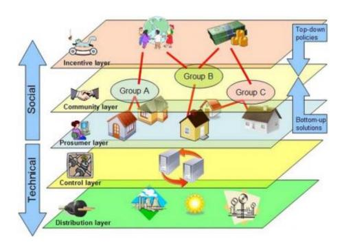
The Energy Web is a power distribution system designed for managing a large-scale, widely distributed network of renewable energy sources. The figure shows the interaction of the different parts of the Energy Web, which includes incentives for "prosumers" (producers and consumers of energy) and allows autonomous self-organization of agents due to evolutionary processes. Image credit: Carreras, et al. ©2010 IEEE.
