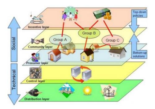
The Energy Web is a power distribution system designed for managing a largescale, widely distributed network of renewable energy sources. The figure shows the interaction of the different parts of the Energy Web, which includes incentives for "prosumers" (producers and consumers of energy) and allows autonomous self-organization of agents due to evolutionary processes. Image credit: Carreras, et al. ©2010 IEEE.
