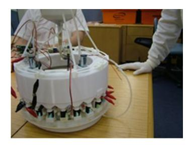
This is the middle section of the robot which consists of the sludge distribution mechanism (white solid helical rings), and the Microbial Fuel Cells (24 in total) which are shown just below the distribution mechanism. Underneath the MFCs there is an overflow collection tray which feeds back into the ingestion vessel above. Image credit: Bristol Robotics Laboratory
