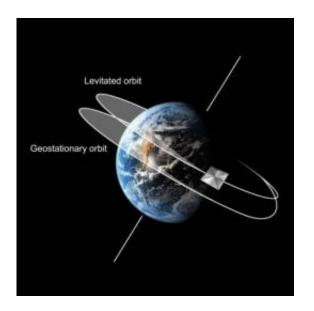
This is a schematic of displaced geostationary orbit. Credit: Advanced Space Concepts Laboratory, University of Strathclyde
