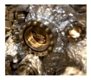
This view provides a look into the heart of a scanning tunneling microscope in the specially designed Princeton Nanoscale Microscopy Laboratory, where highly accurate measurements at the atomic scale are possible because sounds and vibrations, through a multitude of technologies, are kept to a minimum. Credit: Princeton University, Office of Communications, Brian Wilson
