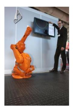
Pressure sensitive flooring detects people and slows or stops the robot's movement. (© Fraunhofer)
