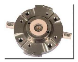
The diamond anvil cell is small enough to fit in the palm of one's hand, but it can compress a sample to extreme pressures up to about 3.6 million atmospheres at room temperature and 1.7 million atmospheres at 3,000 C.
