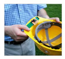
Using only radio waves for its electrical power, the SmartHat has a beeper that alerts the wearer to dangerous construction equipment nearby.
