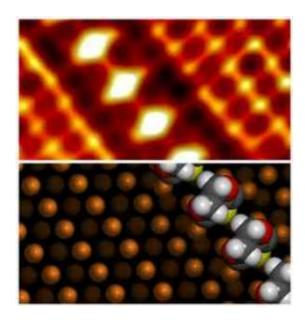
A high-resolution scanning tunneling microscope image (top) and density functional theory-calculated structures (bottom) reveal the formation of a well-organized PEDOT polymer.
