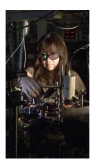
NIST Fellow Deborah Jin in her laboratory at JILA where she studies ultracold atomic gases and their similarities to high-temperature superconductors. The atoms are initially trapped and cooled in a glass cylinder located below the copper coils. Credit: Burrus/NIST
