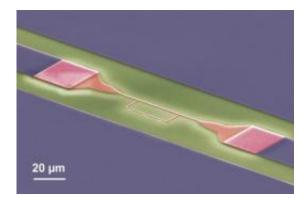
This is an electron microscopical picture of the superconducting circuit (red: Aluminum-Qubit, grey: Niob-Resonator, green: Silicon substrate). Credit: Thomasz Niemczyk, Technische Universitaet Muenchen
