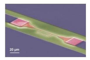
This is an electron microscopical picture of the superconducting circuit (red: Aluminum-Qubit, grey: Niob-Resonator, green: Silicon substrate). Credit: Thomasz Niemczyk, Technische Universitaet Muenchen
