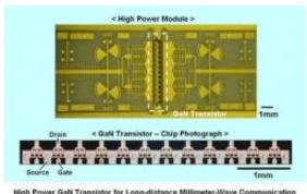
High Power GaN Transistor for Long-distance Millimeter-Wave Communication
