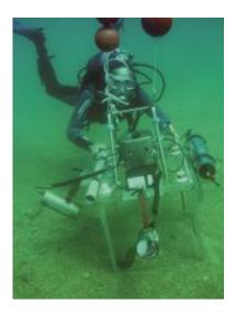
Marine Biology "in situ": A team of scientists explores marine bottom dwellers during oxygen crises with the purpose-built underwater-chamber EAGU (Experimental Anoxia Generating Unit).
