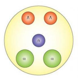
A schematic diagram of a double-hyperon beryllium nucleus. The usual 11 particles of this nucleus have been approximated to two helium nuclei ( $\alpha$ ) (each with two protons and two neutrons, one neutron (n) and two hyperon particles ( $\Lambda$ ) to simplify theoretical calculations of their interactions. © 2010 Emiko Hiyama
