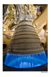
Testing of the Common Extensible Cryogenic Engine, also known as CECE, at 100 percent power level. (NASA/PWR)
