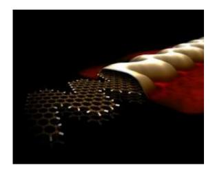
This is a structural model and three-dimensional picture of the scanning tunneling microscope view of a zig-zag shaped graphene nanoribbon. Credit: Empa
