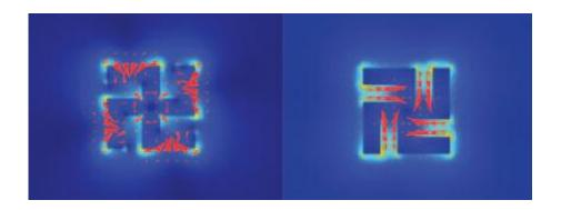
Optical forces induced on a light mill motor by an illumination wavelength of 810 nanometers (left) and 1,700 nanometers. At 810 nm wavelength, light impacts the outer side of the arms, inducing a counterclockwise torque on the motor. At 1,700 nm, light passes through the gaps and impacts the elbow of the motor, providing a clockwise torque. (Image courtesy of Zhang group)
