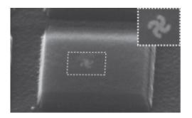
This STM image shows a gammadion gold light mill nanomotor embedded in a silica microdisk. Inset is a magnified top view of the light mill.
