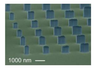
This is a colorized micrograph of semiconductor nanowires grown at NIST in a precisely controlled array of sizes and locations. Credit: K. Bertness, NIST
