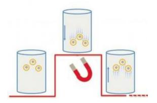
An external magnetic field attracts the nanoparticles by their magnetic cores.
