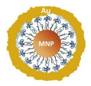
The 30-nanometer particle consists of a magnetic core and a thin gold shell, analogous to an eggshell, that surrounds but does not touch the center. Credit: Xiaohu Gao, University of Washington
