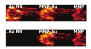
On top are photoacoustic images taken for gold nanorods (left), the new UW particle that has a magnetic core and surrounding gold shell (center), and a simple magnetic nanoparticle (right). Below is the same image after processing to remove pixels not vibrating with the magnetic field. The center blob is retained because of the particles' magnetic core and is bright because of the particles' gold shell. Credit: Xiaohu Gao, University of Washington
