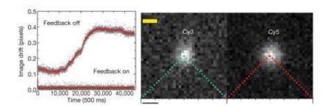
The graph on left shows that with the active feedback system off there is a resolution drift of about 0.3 pixels or 19 nanometers, but with the feedback system on resolution is maintained at better than 0.01 pixels, or about 0.64 nanometers. The image on right shows individual Cyanine (Cy) fluorescent dye molecules -- Cy3 and Cy5 -- used to label 20 base pairs of double-stranded DNA. Credit: Courtesy of Steven Chu research group
