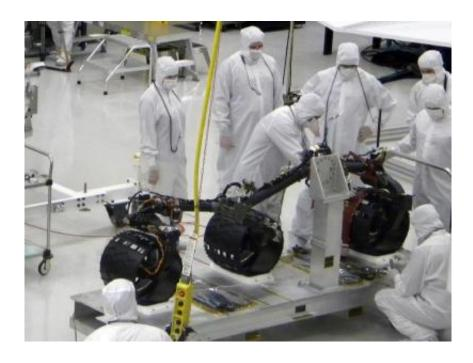
With the wheels and suspension system already installed onto one side of NASA's Mars rover Curiosity the previous day, spacecraft engineers and
