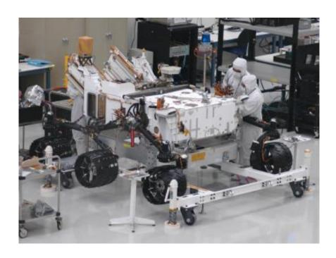
Mars rover Curiosity, the centerpiece of NASA's Mars Science Laboratory mission, is coming together for extensive testing prior to its late 2011 launch. Image Credit: NASA/JPL-Caltech
